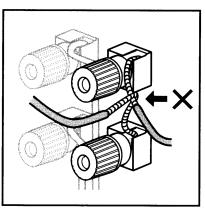
Make sure that exposed speaker wire does not extend outside the speaker terminal and touch any other wire.
